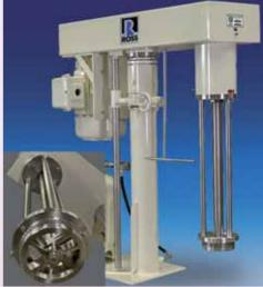
Figure 3 – PreMax Batch Ultra-High Shear Mixer with "Delta" rotor/stator (US Patent No.6,000,840) capable of tip speeds up to 5000 ft/min (1524 m/min).
